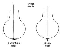
flasks greatly improves this situation, though smooth stirring with normal octagonal stir bars is difficult with these flasks. Although special stir bars have been designed to cope with this problem, it would be more convenient if one could use regular octagonal stir bars.
